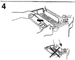
If the paper is jammed within the fusing unit, grasp the bottom part of the paper and pull down as shown.
