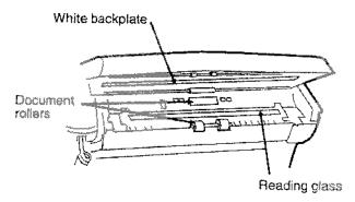
Wipe the reading glass, white backplate, and rollers with a soft cloth.
