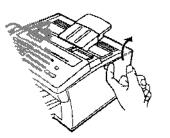
Open the printer cover at the rear of the fax by grasping the finger hold on the right side of the cover and pulling up.
