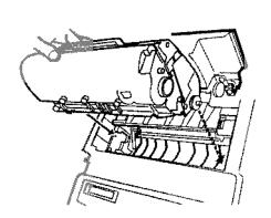
insert the cartridge into the fax as shown, using the cartridge guides to position it properly. Push down gently on the cartridge to ensure that it is well seated.
