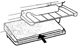
Place the paper cover on the paper tray so that the guides go inside the cover, and slide the cover in.
