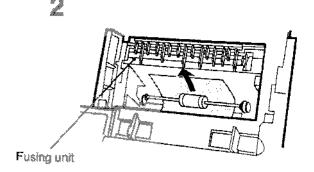
If the edge of the paper has not entered the fusing unit, remove the paper by pulling up as shown.
