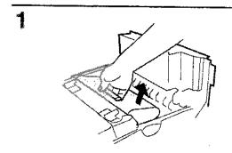
Open the printer cover and remove the imaging cartridge.
