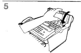
Replace the imaging cartridge and close the printer cover.
