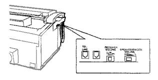
Adjust the volume switches on the left side of the fax:
