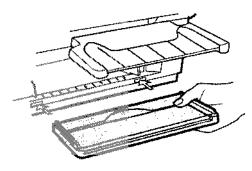
Attach the paper tray by inserting the tabs into the holes at the bottom of the fax.
