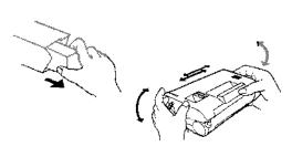
Remove the imaging cartridge from its box. Hold it with both hands, and shake it well in the directions shown.
