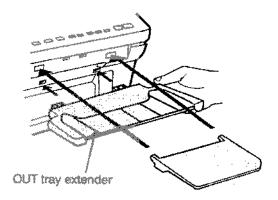
Attach the original document guide by inserting the tabs into the holes at the top of the fax.
