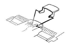
Attach the IN tray extender to the original document IN tray by inserting the tabe on the ends of the extender into the holes in the sides of the tray.
