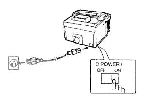
Plug the female end of the power cord into the power socket on the back of the fax. Plug the male end into a 120 V, 60 Hz, grounded (3-prong) outlet.
