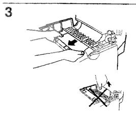
if the leading edge of the paper has entered the fusing unit, first remove the leading edge from the fusing unit by pulling down as shown, then remove the entire sheet by pulling up as shown in Step 2.
